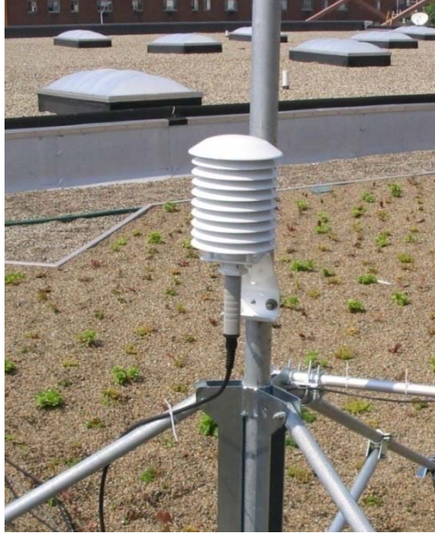
Figure 3-3 Relative humidity sensor for recording ambient air temperature and relative humidity in radiation shield (Giant Eagle)
