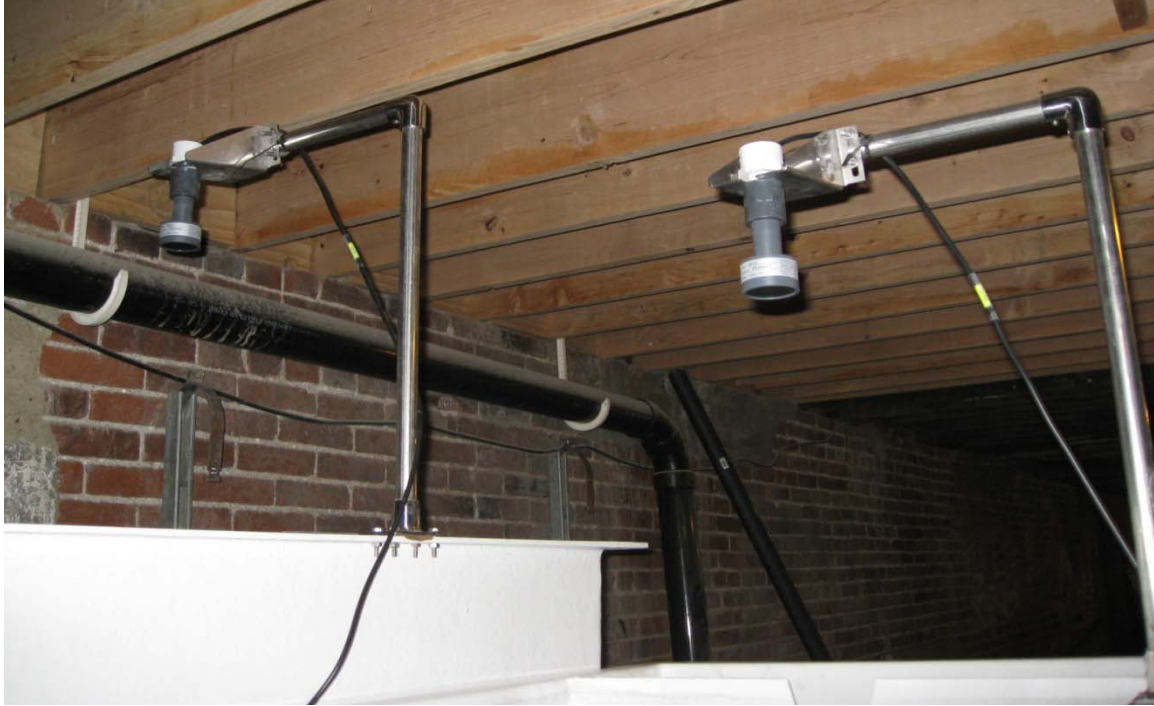
Figure 3-19 Ultrasonic sensors monitored changes in water level over weirs at the Homestead Site.
